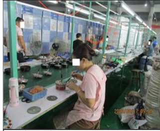
Photo of non-conformity Tin-soldering worker not provided with dust proof mask and no LEV system for tin-soldering.JPG
