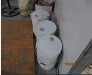
Photo of non-conformity Diffusion oil without label and not stored in secondary containment.JPG
